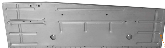
520188 LATERAL FLOORPANEL LEFT 69+ REINFORCE (1,2 mm)
